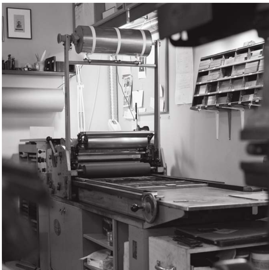
The Vandercook Universal III printing press in the Lumiere Press workshop.
